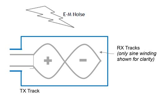
The main RX tracks with one sin/cos cycle per rev defines absolute position. A secondary track with multiple cycles enhances resolution. More typically the main TX track has multiple cycles (9 for example) combined with a secondary track with a number of cycles not a multiple of 3 – every position within one rev is defined by two unique readings.
