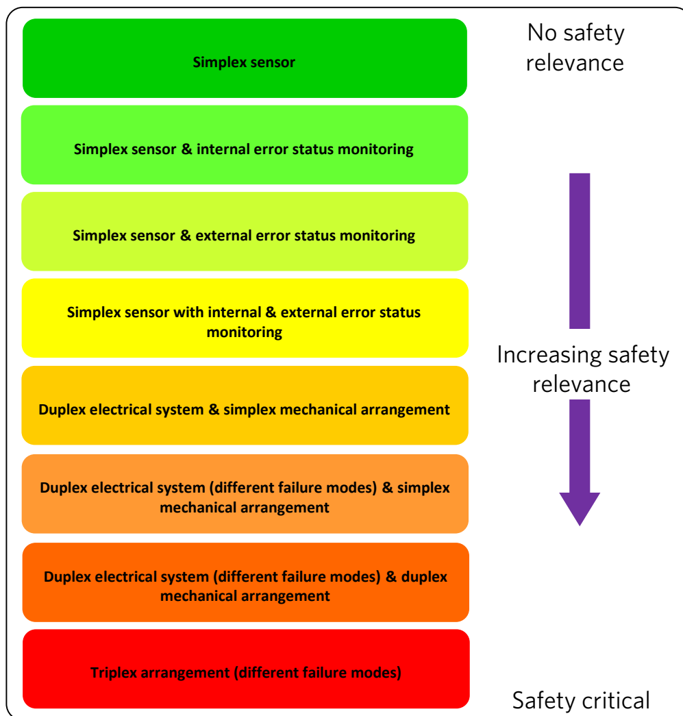
Figure 1. A spectrum of design approaches for position sensors as safety demands increase
