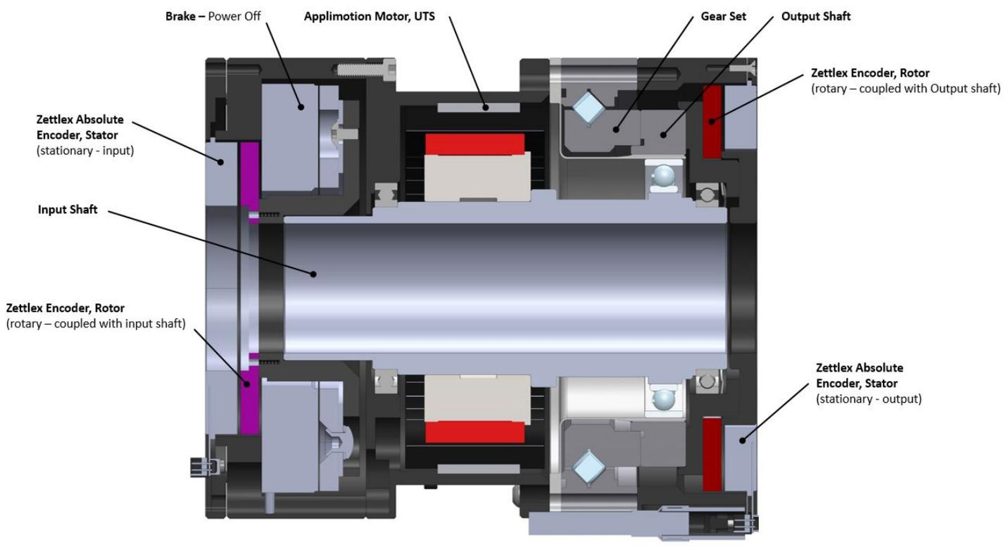
The above cross-section defines the major components of a Celera Motion dual encoder robot joint. The components include:
